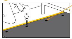
fasten at the front edge through the prefabricated fastening points
